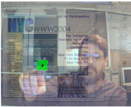
Figure 5. Facetop at semi-transparent level with finger tip tracking marked green. [18]
